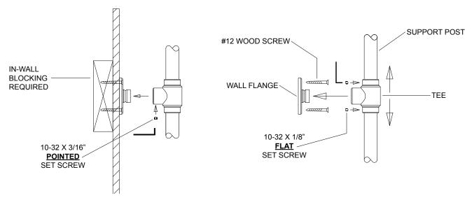
SECURE THE SUPPORT POSTS TO THE WALL FLANGES. THE TEES MAY BE ADJUSTED SLIGHTLY TO HELP LOCATE ONTO THE WALL FLANGES. IT IS IMPORTANT THAT THE TEES ARE SECURED TO THE WALL FLANGES USING THE PROVIDED 3/16" POINTED SET SCREWS.
