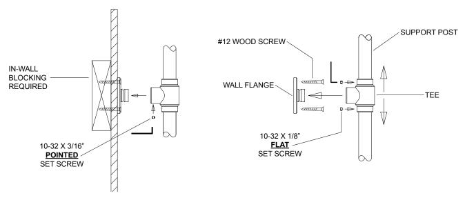
SECURE THE SUPPORT POSTS TO THE WALL FLANGES. THE TEES MAY BE ADJUSTED SLIGHTLY TO HELP LOCATE ONTO THE WALL FLANGES AND TO POSITION THE CEILING FLANGES. IT IS IMPORTANT THAT THE TEES ARE SECURED TO THE WALL FLANGES USING THE PROVIDED 3/16" **POINTED** SET SCREWS.
