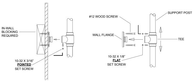
SECURE THE SUPPORT POSTS TO THE WALL FLANGES. THE UPPER TEE MAY BE ADJUSTED SLIGHTLY TO HELP LOCATE ONTO THE WALL FLANGES. IT IS IMPORTANT THAT THE TEES ARE SECURED TO THE WALL FLANGES USING THE PROVIDED 3/16" POINTED SET SCREWS.
