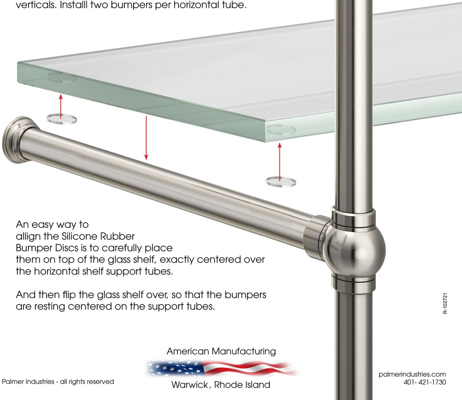
An easy way to align the Silicone Rubber Bumper Discs is to carefully place them on top of the glass shelf, exactly centered over the horizontal shelf support tubes.
