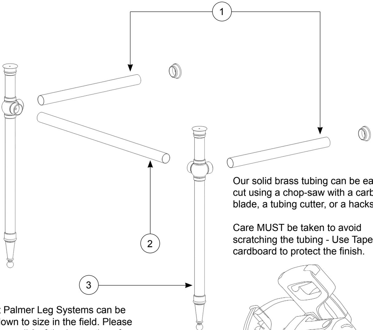
Our solid brass tubing can be easily cut using a chop-saw with a carbide blade, a tubing cutter, or a hacksaw.
