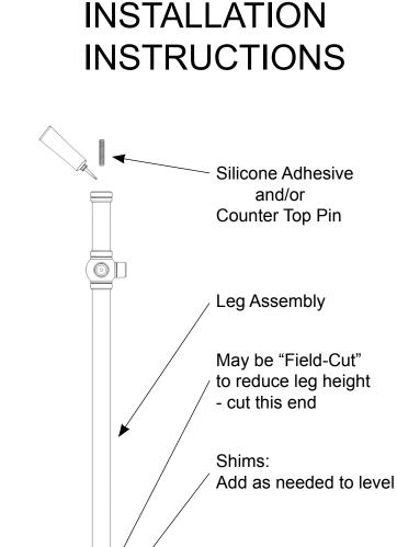
Floor Pins MUST engage 1/4"diameter holes drilled into flooring. Recommended minimum hole depth of 1/4"
