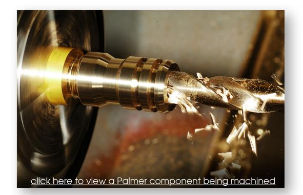
Our components are proprietary to Palmer, precision machined from solid brass rod with computer-controlled equipment, producing a perfect fit and finish consistent with the highest-quality bath furniture.
