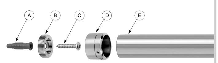
1. Locate and attach Threaded Plug (B) to wall using Wall Anchor (A) and Structural Screw (C)
