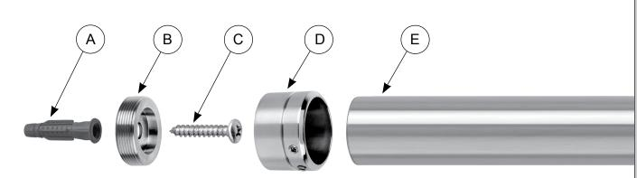
1. Locate and attach Threaded Plug (B) to surface using Plastic Anchor (A) and Structural Screw (C).
