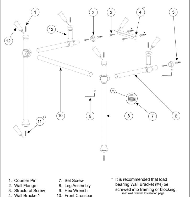
\*\* Floor Pins (#11) MUST engage 1/4" diameter holes drilled into flooring
