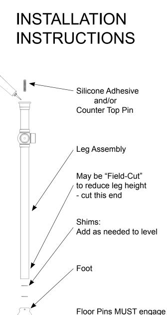
1/4"diameter holes drilled into flooring. Recommended minimum hole depth of 1/4"
