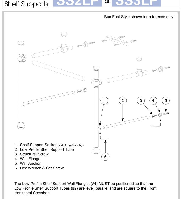
\* Note: For Leg System Configurations with rear Legs, the Low-Profile Shelf Support Tubes (#2) are connected to the Shelf Support Sockets (#1) on the front and rear legs.
