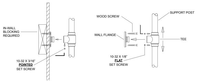
SECURE THE SUPPORT POSTS TO THE WALL FLANGES. THE UPPER TEE MAY BE ADJUSTED SLIGHTLY TO HELP LOCATE ONTO THE WALL FLANGES. IT IS IMPORTANT THAT THE TEES ARE SECURED TO THE WALL FLANGES USING THE PROVIDED 3/16" POINTED SET SCREWS.
