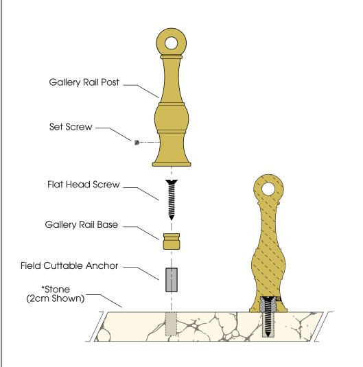
\*Ø7/32" Hole x 5/8" Depth Required For Anchor
